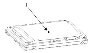
Figure 3.5 Surface cover temperature measurement points
